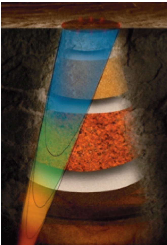
Figure 3. PanGeo Subsea's Acoustic Zoom technology is an example of the next generation of geophysical technologies. The deep earth telescope is theoretically capable of generating high resolution acoustic images five to 10 times greater than conventional 3D and 4D seismic (source: PanGeo Subsea).
